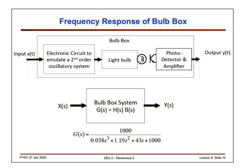
Let us now apply what we have learned in this Lecture to Lab 2 experiment using the Bulb Box. The box has an electronic circuit which behaves like a second-order system with a natural frequency of 5Hz and a very low damping ratio (i.e. highly oscillatory). The output of this circuit drives the light-bulb and photo-diode circuit to produce an output depending on the light intensity.
